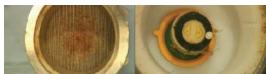
Figure 1. Failure of H 2 S sensors caused by hose down
