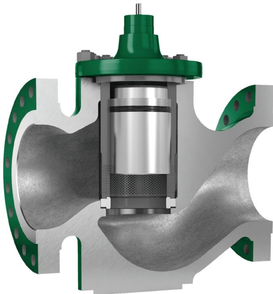
Figure 5. Special valve trims, such as the Emerson Fisher Whisper III trim, can be employed to attenuate noise, reduce cavitation, or direct cavitating liquids away from valve components—all of which minimize damage to the valve.
