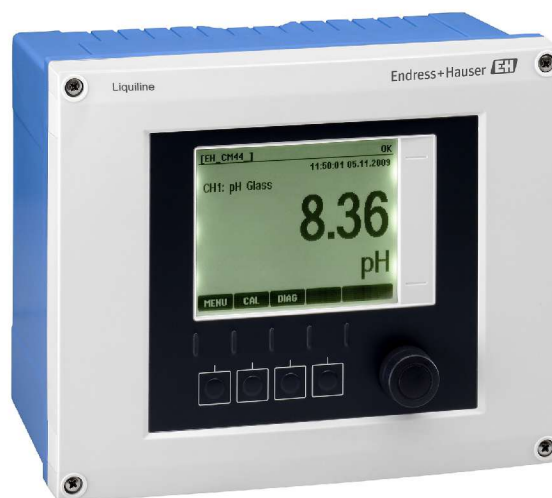
Figure 1. Information can now be communicated bidirectionally between instruments and control systems, dramatically improving the way companies operate a process and manage assets. The Liquiline transmitter is an example, communicating via EtherNet/IP, Modbus RS485, or TCP, PROFIBUS DP, and HART as well as a web server.
