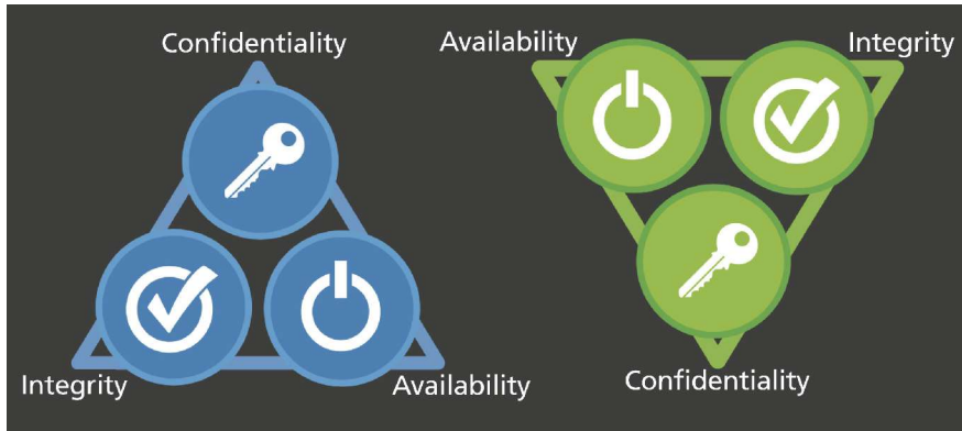
Figure 1. The triads representing the areas of concern for IT (on the left) and OT (on the right) are becoming less distinct as technologies and responsibilities become more similar. Source: Cisco
