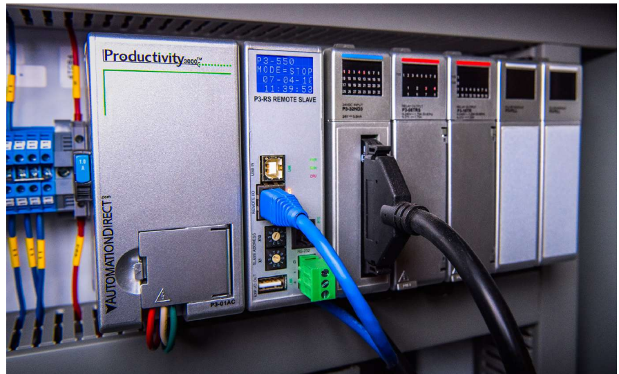
Figure 2. Modern controllers, such as this AutomationDirect Productivity3000, have data handling capabilities, including built-in data logging, and communication features for remote monitoring via email, web browsers, and mobile apps.
