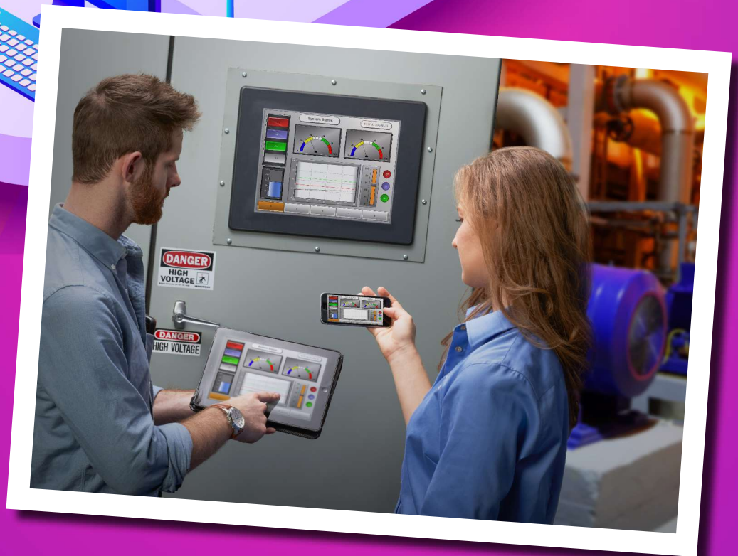
Figure 1. HMI remote access: This C-more HMI touch panel provides remote access functionality, as well as local control and monitoring.
