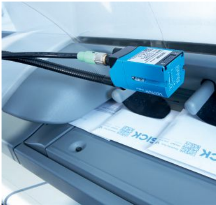
Vision sensors can verify the correct code was used and that it actually printed.
