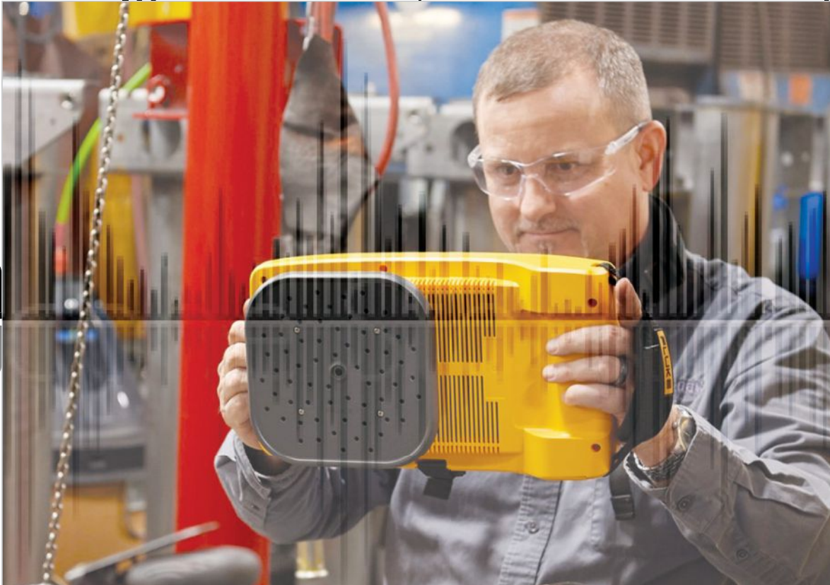
An array of tiny supersensitive microphones on a sonic imager detects sounds outside the range of human hearing.
