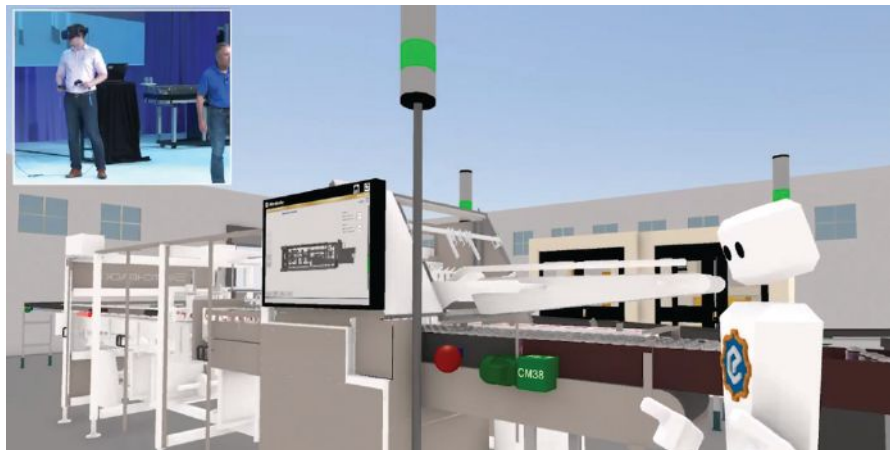
The operator within the XR model can move around within the model by teleporting, and can be teleported by another user. Both can interact with controls and products using the handheld controllers, and they see each other as avatars within the model.
