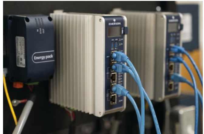
Figure 4. Edge controllers are built for field installation, and are an ideal platform for integrating OT data with IT analytical computing close to the data sources.
