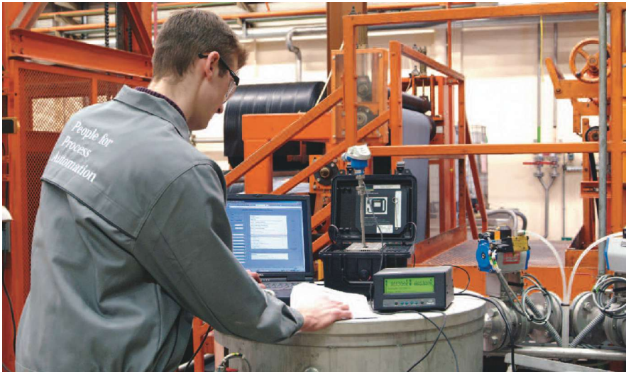
Some asset management systems allow access to instrument information by mobile devices. This maintenance technician gets the data he needs to troubleshoot the level instrument on this tank.
