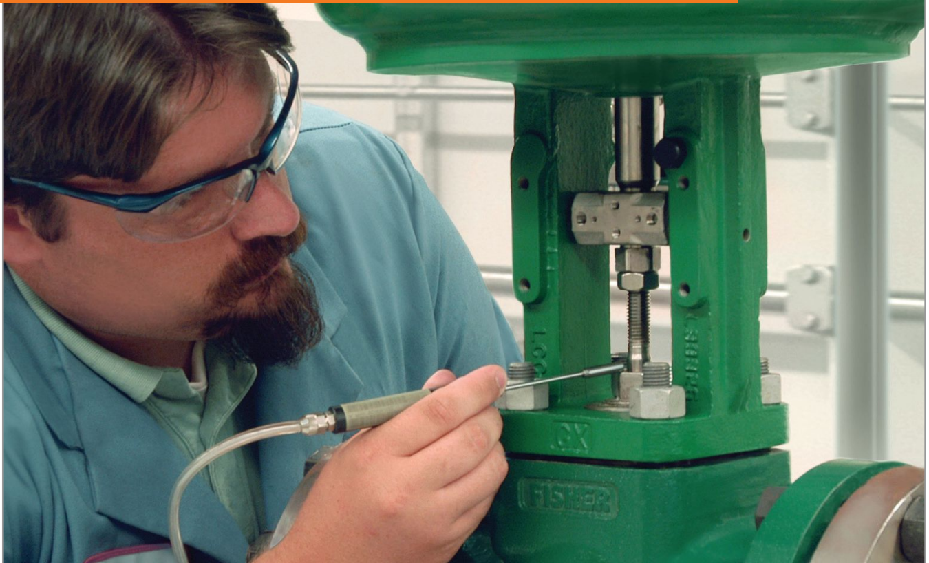
Figure 1. This control valve is subjected to EPA's Method 21 "sniff" test to determine the fugitive emission leak rate after a prescribed number of mechanical and thermal cycles.
