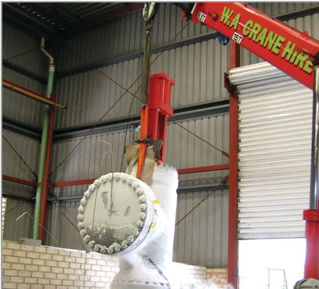
Figure 5. This 24-inch by 30-inch letdown valve employs a specially designed large stem diameter environmental seal for extremely low leakage rates, as demonstrated here during a test at -56^{\circ}\text{F} .
