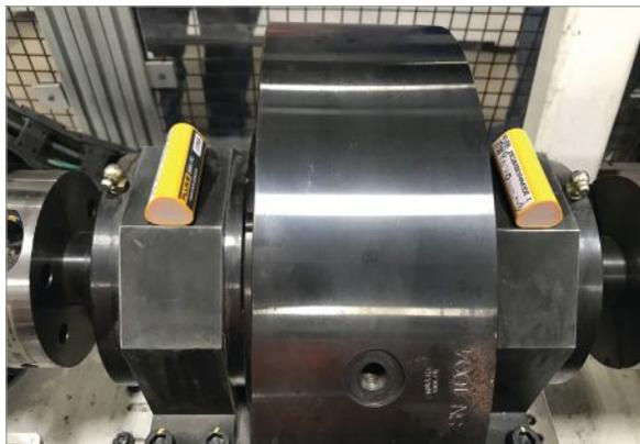
Vibration and power monitoring sensors attached to manufacturing plant machinery, shown in yellow, provide continuous streams of condition data.
