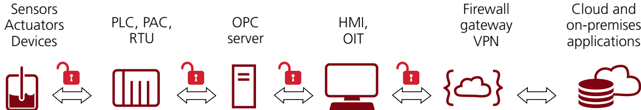
Figure 1. Traditional industrial communications architectures have demanded many layers of hardware and software, driving up cost and complexity and driving down performance.
