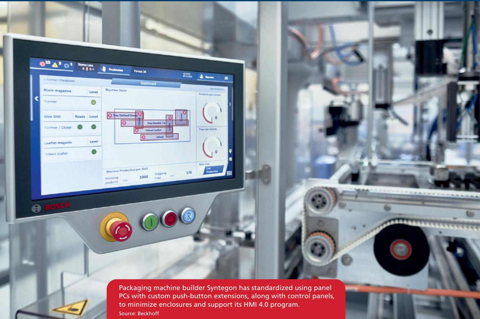
Packaging machine builder Syntegon has standardized using panel PCs with custom push-button extensions, along with control panels, to minimize enclosures and support its HMI 4.0 program.
