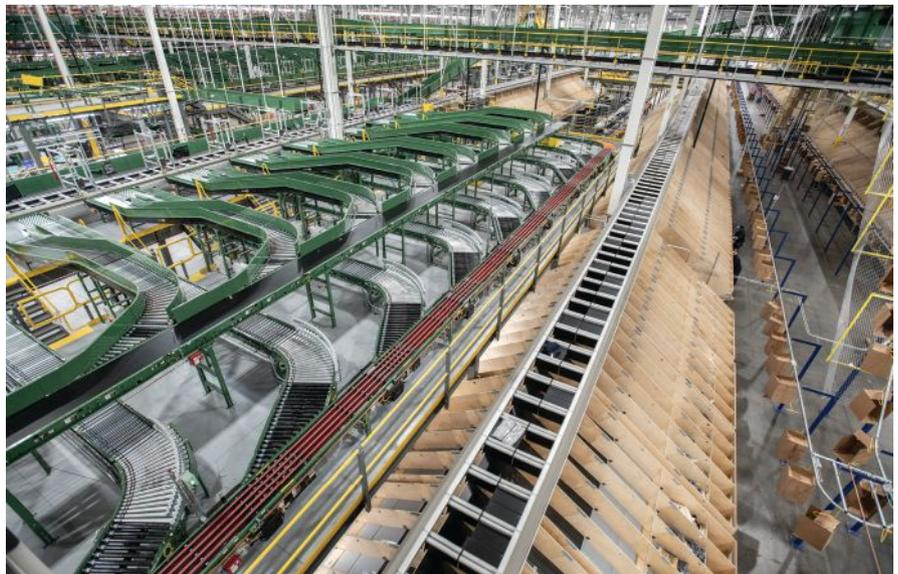
EuroSort used elements of cabinetless design in the distribution center redesign for Gap, Inc., which optimized space, performance, and cost.
