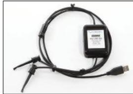
It is the lowest cost USB Modem certified by the FieldComm Group to meet the HART communication specifications.
