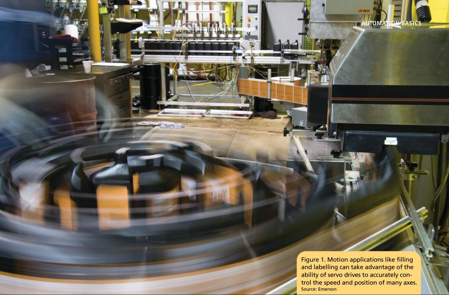
Figure 1. Motion applications like filling and labelling can take advantage of the ability of servo drives to accurately control the speed and position of many axes.
