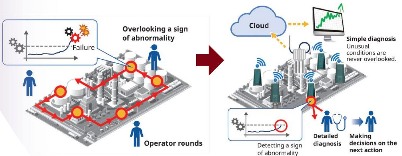
Figure 1. An operator following a prescribed route to check equipment is costly and time consuming, and not nearly as effective as automated condition monitoring.
