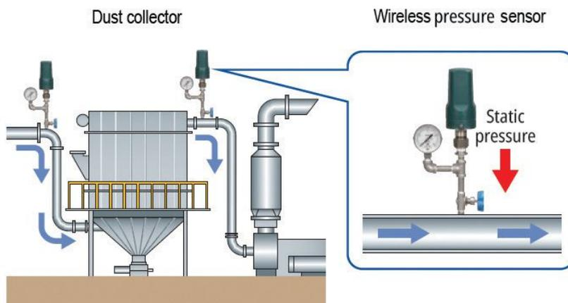
Figure 3. Sensors like Yokogawa's Sushi Sensor can provide a pressure measurement via LoRaWAN at the outlet of a bag house to indicate if it is clogged or if it is leaking due to torn bags.
