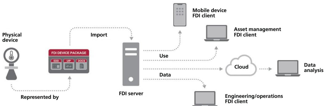
Figure 1. FDI takes the best features of EDDL and FDT packages and combines them into a single common standard, simplifying installation and reducing or eliminating device compatibility concerns.
