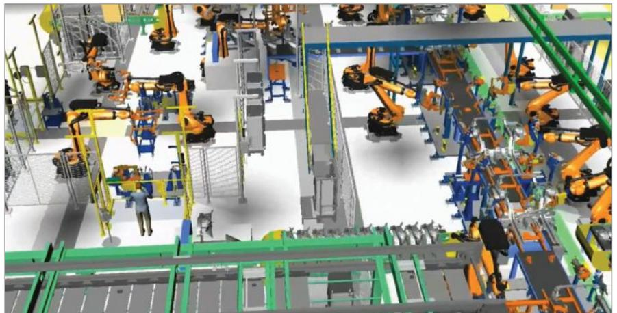
Figure 4. One manufacturing company optimized operations and predicted throughput with more than 99 percent accuracy using Siemens digital twin methodology with Plant Simulation and MindSphere applications.
