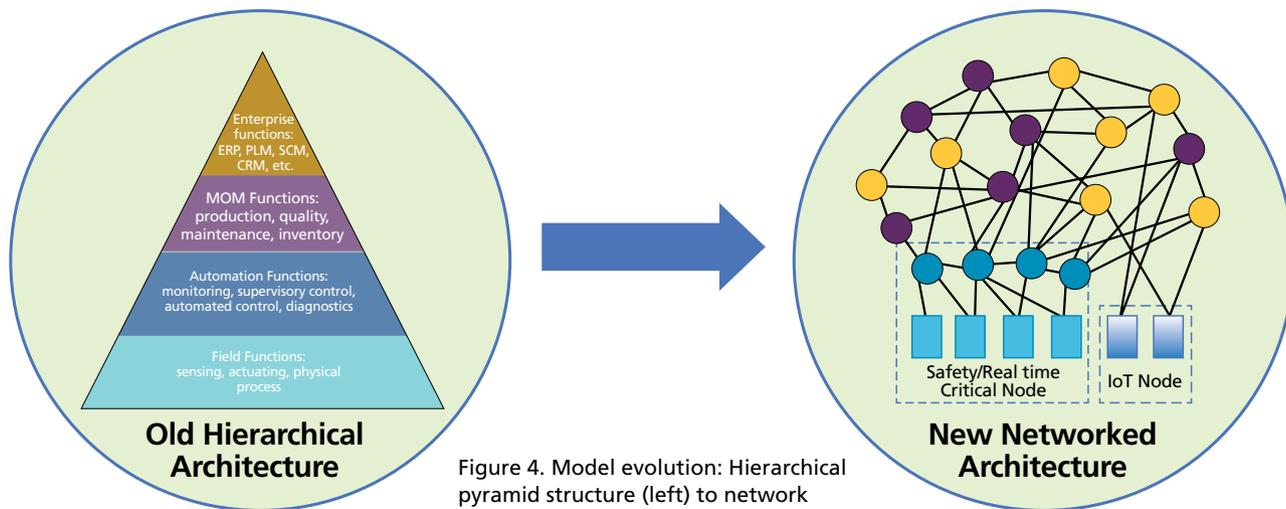
Figure 4. Model evolution: Hierarchical pyramid structure (left) to network structured architecture (right).
