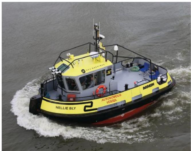
Autonomous operations come to the open ocean with Sea Machines' SM300 system, which uses computer vision and augmented reality. See page 13.
