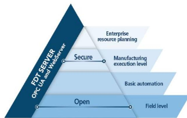
FDT 3.0 provides the industrial enterprise with native integration of the OPC Unified Architecture (OPC UA), as well as control and web services interfaces for mobile applications.
