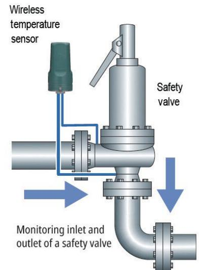
Figure 4. Measuring the temperature differential on both sides of a PRV with a Yokogawa Sushi Sensor communicating via LoRaWAN can indicate when it is firmly closed or is leaking.
