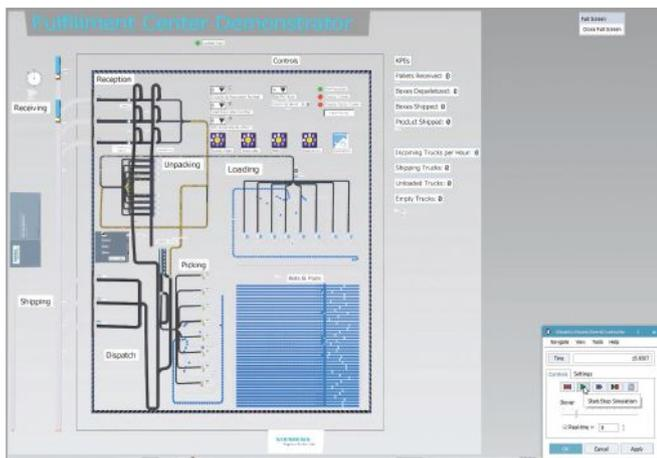
Figure 1. Users can adjust control parameters in software like Siemens Plant Simulation to visualize and determine effects on throughput and other KPIs.
