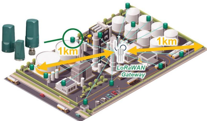
Figure 2. LoRaWAN is well suited to supporting a wide-area network of condition-monitoring sensors, concentrating all the relevant data in one place.
