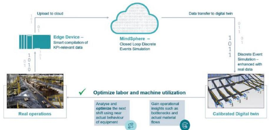
Figure 3. An open IoT cloud platform, such as Siemens Industrial Edge and Cloud native apps, empowers users to calibrate their digital twin with historical production data.
