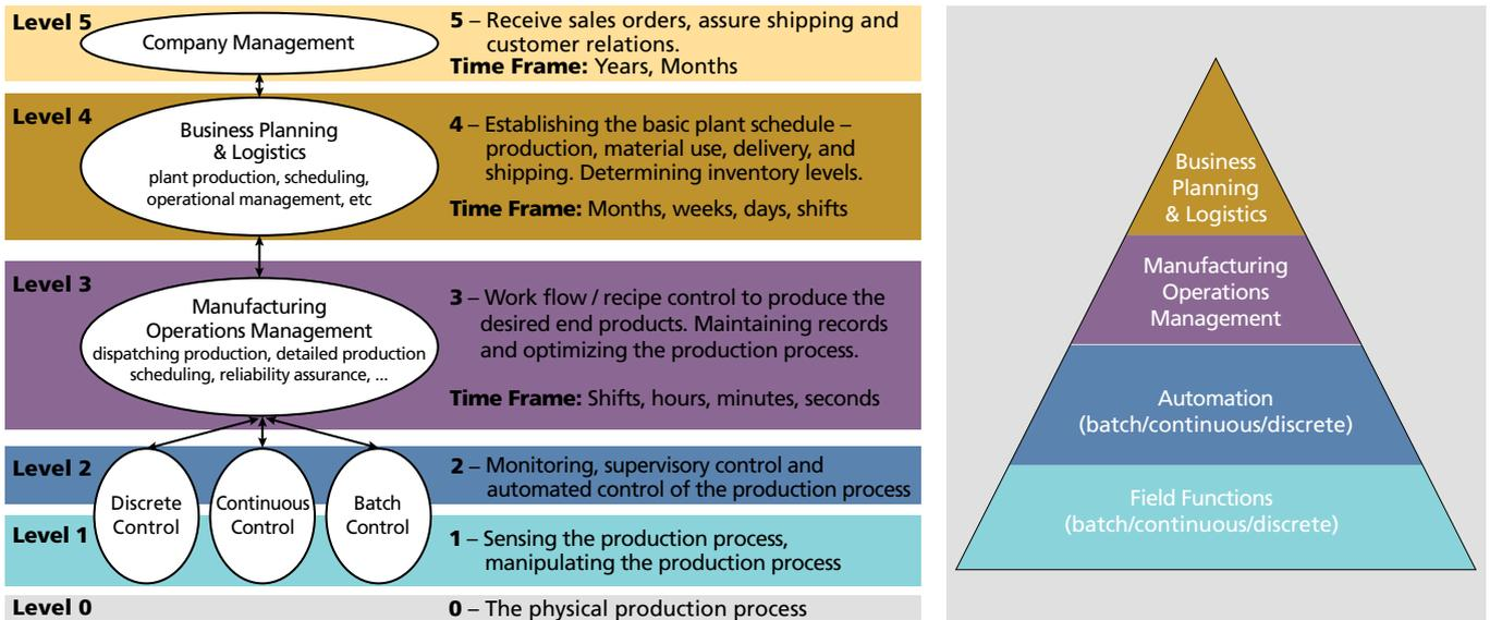
Figure 2. The ISA95 functional model (left) is more traditionally presented as a pyramid.
