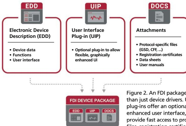
Figure 2. An FDI package contains more than just device drivers. User interface plug-ins offer an optional graphically enhanced user interface, and attachments provide fast access to protocol-specific files, registration certificates, data sheets, and manuals.
