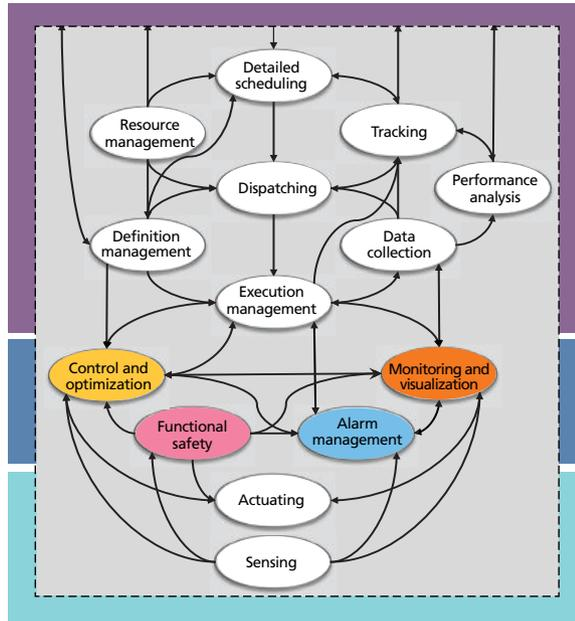
Figure 6. This networked reference architecture for operations in a manufacturing organization is an extension of the ISA95 Activity model. Each oval represents an activity as a set of tasks.
