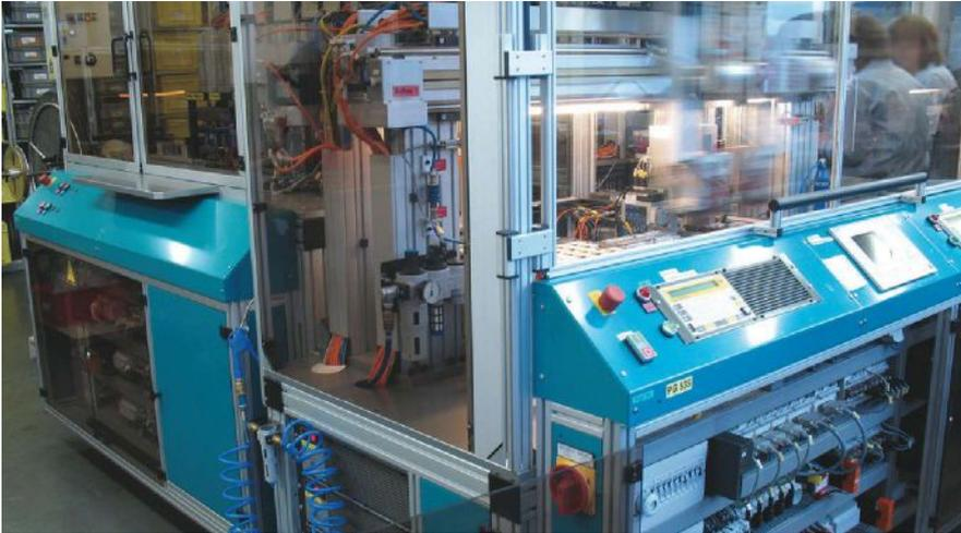
Figure 4. Advanced safety relays or safety controllers are more suitable for more complicated moving equipment installed within a guarded cell.
