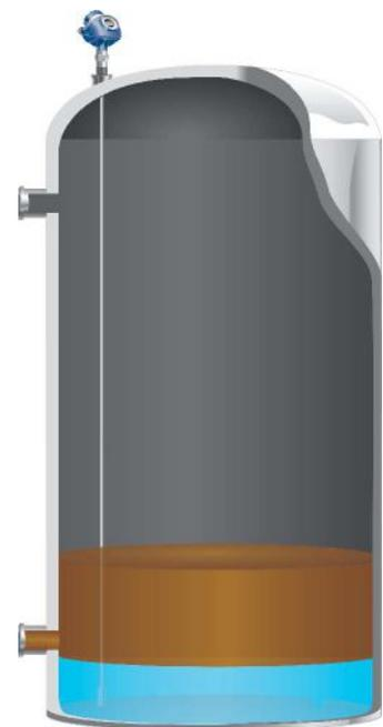
Figure 2. A guided wave radar (GWR) instrument uses a metallic probe to guide the pulse to the surface and back. (Shown is a Rosemount 5300 Level Transmitter.)
