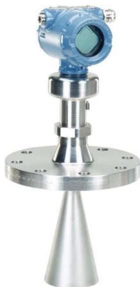
Figure 3. A frequency-modulated continuous wave (FMCW) instrument delivers more powerful reflections to provide a higher degree of accuracy than most pulse-based radar transmitters. (Shown is a Rosemount 5408 Level Transmitter.)
