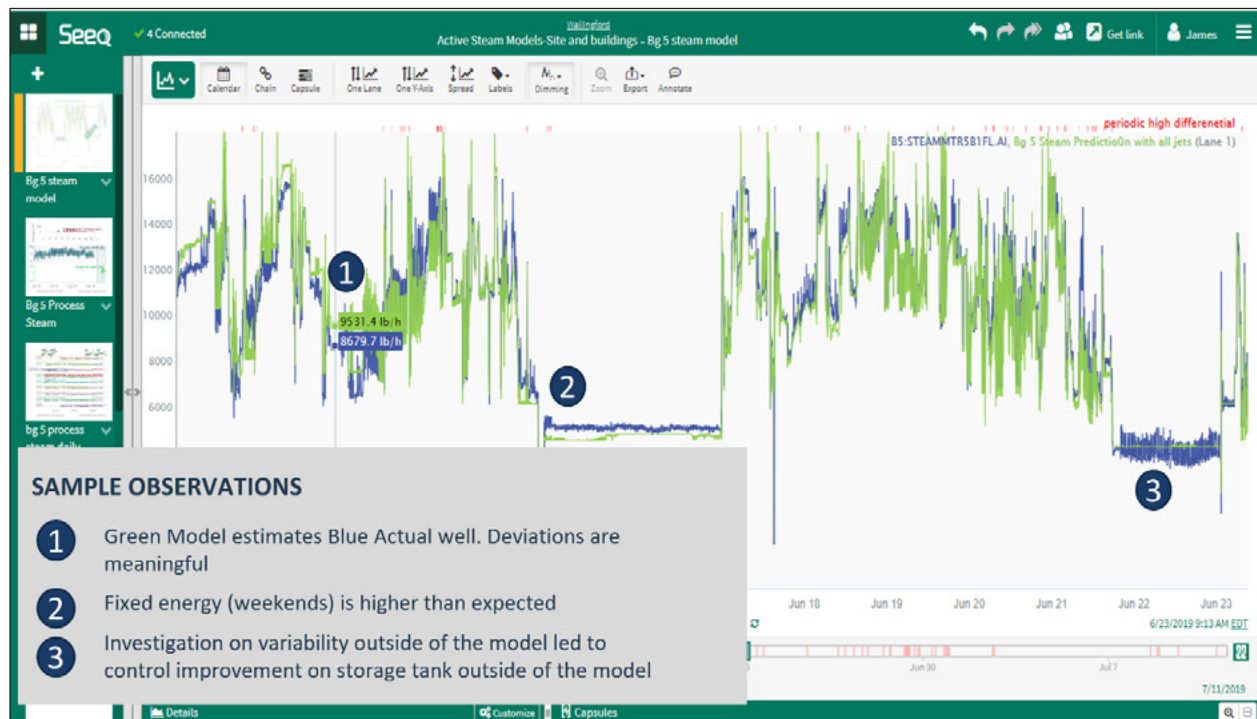
Figure 1. Using advanced analytics, companies can model the impacts of operational modifications on such process variables as energy consumption to determine optimal conditions.
