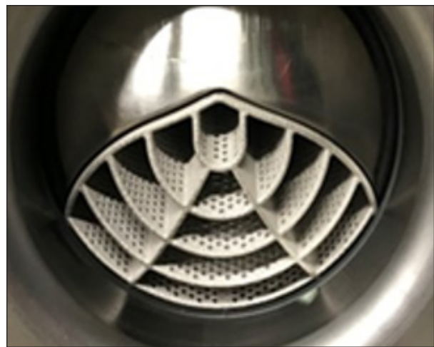
Figure 3. Innovative additive manufactured rotary valve solutions can reduce sound levels up to 80 percent over traditional manufactured designs.
